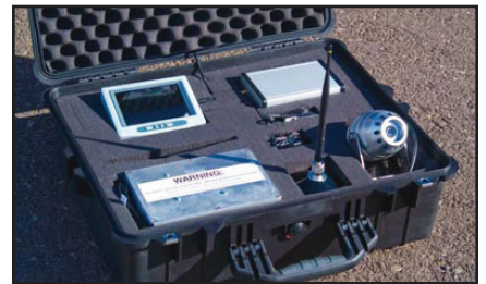
▲ TRACS' wireless camera system comes securely packaged in a Pelican case that houses monitor during operation. Photo: Northern Lights Tactical
